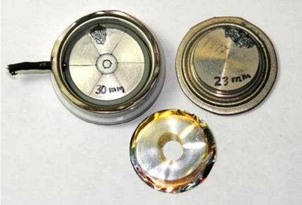
**Figure 3.** 30mm Power Thyristor Pellet and Case
